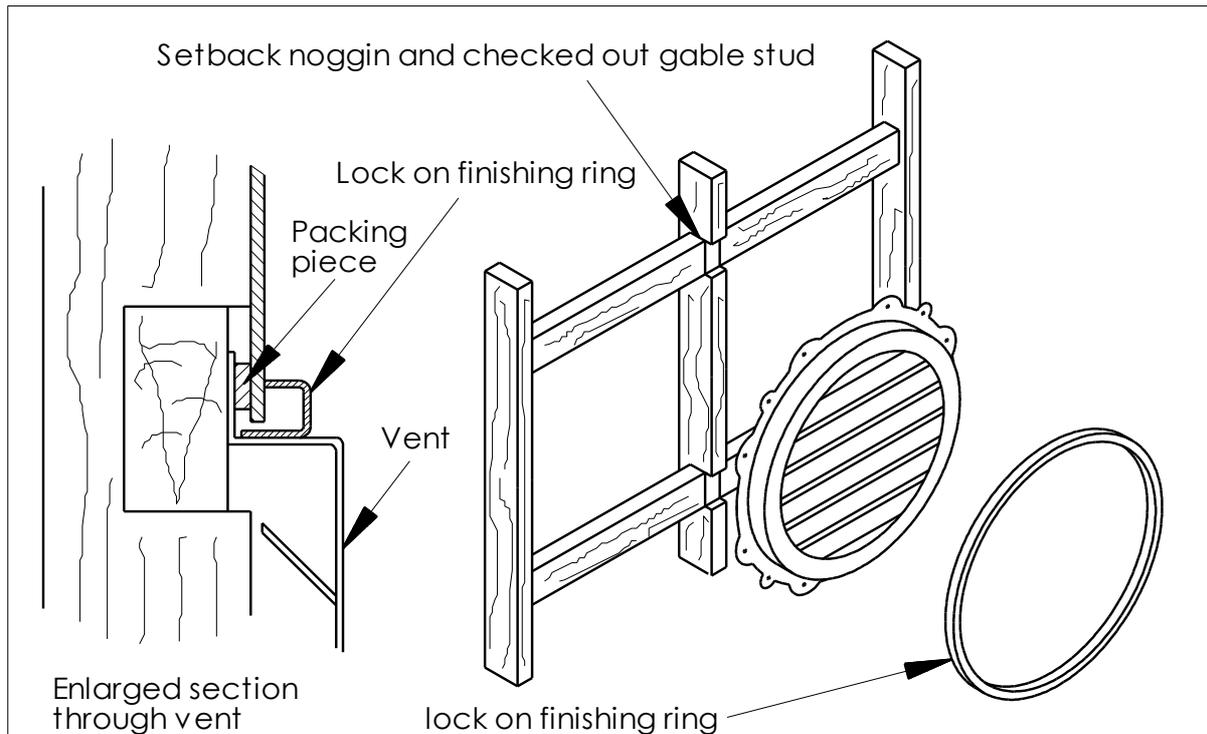
**Due to thickness of this cladding, it is necessary to use noggins set back from the front face of the gable studs.**
